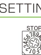
Idle Current (STOP : Rotary Switch)
